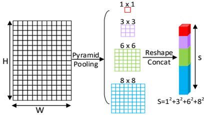
Figure 3. Illustration of the pyramid average pooling process.
