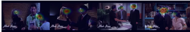
Figure 7: Constructed shared attention map obtained by adding up individual heatmaps of all people in the image. Samples are from the VideoCoAtt dataset.
