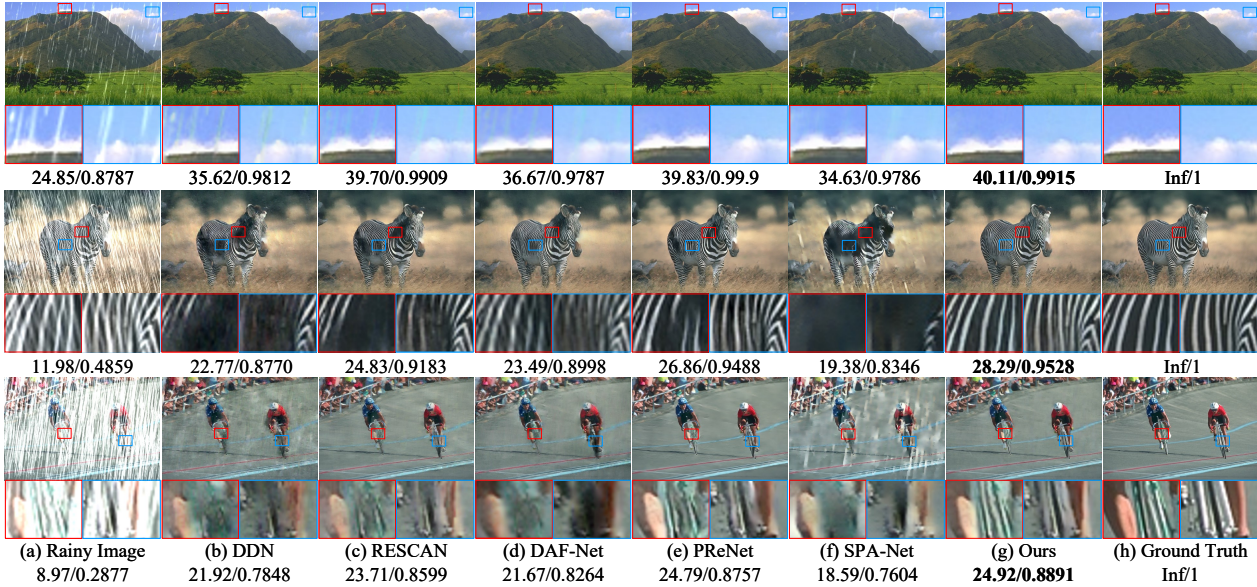
Figure 5. Image deraining results tested in the synthetic datasets. From (a)-(h): (a) the rainy images, and the deraining results of (b) DDN [5], (c) RESCAN [16], (d) DAF-Net [10], (e) PReNet [21], (f) SPA-Net [25], (g) our DRD-Net respectively, and (h) the ground truth.
