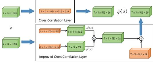
Figure 3. The architecture of the vanilla and improved cross-correlation layers. Green cubes denote the feature maps and orange ones denote the parameters to learn. “ $\otimes$ ” denotes outer product and “ $\oplus$ ” denotes element-wise sum.
