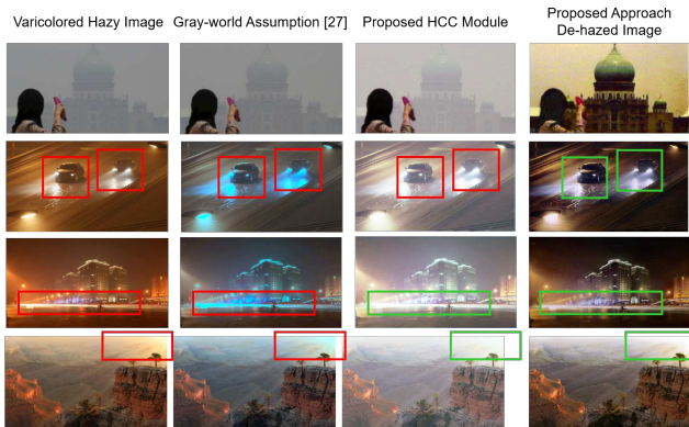
Figure 4. Restoration of the color balance in varicolored hazy image
