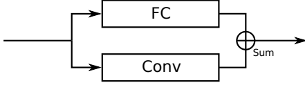
Figure 2: Our block learns the sum of one graph convolution and a shortcut equipped with an affine transformation.
