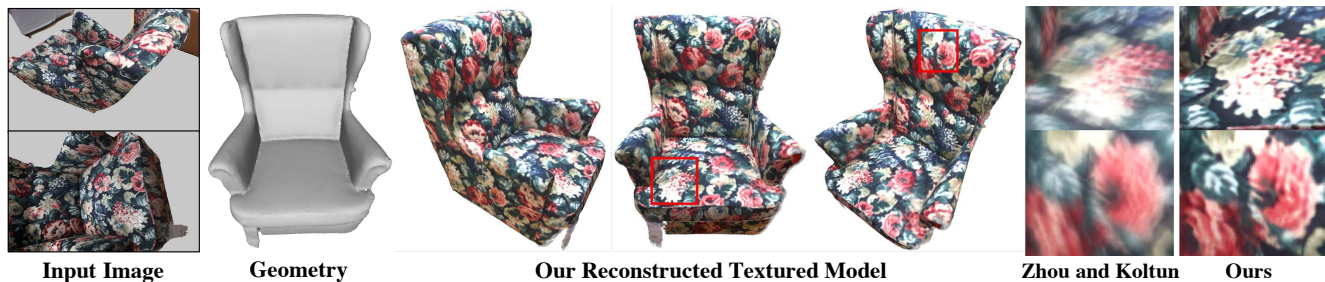
Figure 1. Our goal is to reconstruct high-quality textures from an RGB-D scan. Unlike traditional methods which optimize for a parametric color map to reduce misalignment error (Zhou and Koltun [36]), we learn a misalignment-tolerant discriminator, producing sharper textures.
