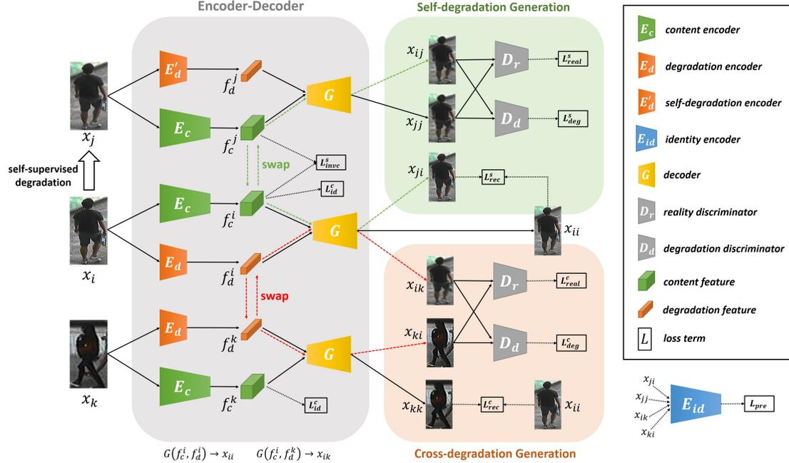
Figure 2. Overview of the proposed Degradation Decomposition Generative Adversarial Network, DDGAN. A self-degraded image pair  $\{x_i, x_j\}$  and a real image pair  $\{x_i, x_k\}$  are alternately used to train the DDGAN. For each pair, input images are decomposed into content features  $f_c$  and degradation features  $f_d$ , which are then swapped and combined to generate four reconstructed images, e.g.,  $\{x_{ii}, x_{ij}, x_{ij}, x_{ji}\}$ .
