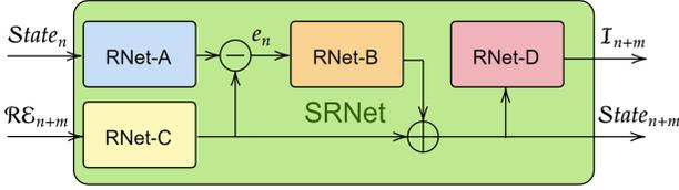
Figure 4. Detailed architecture of the proposed super resolving network (*SRNet*) (Green-block in Fig. 2). Four main residual networks are designed to perform as a large encoder-decoder scheme. *RNet-A* is used to update the hidden state while *RNet-B* and *RNet-D* act as an encoder and decoder respectively to map the hidden state as a super resolved intensity output ( $I_{n+m}$ ).
