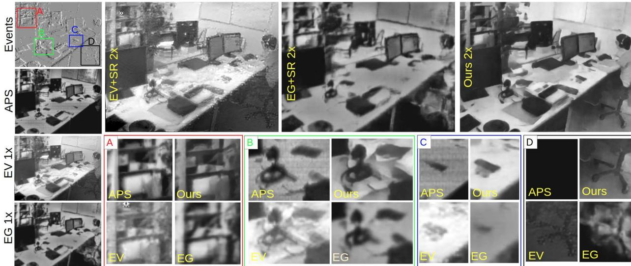
Figure 1. Reconstructing high-definition photo-realistic intensity images from pure events in end-to-end learning. Our events to super-resolved intensity image reconstruction recovers more details with less artifacts in comparison to recent methods of EG [24] and EV [17].
