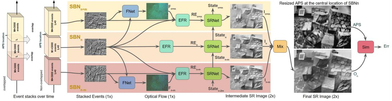
Figure 3. Detailed data flow in the proposed method. This example is based on third stack ( $SBN_{n+m}$ ), therefore the previous inputs, optical flow, and intermediate intensity outputs are faded. The APS frame is resized to the size of output ( $O_n$ ) for comparison
