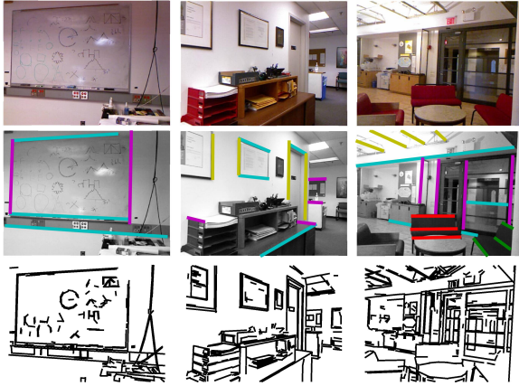
Figure 3: Examples from our newly presented NYU-VP dataset with two (left), three (middle) and five (right) vanishing points. Top: Original RGB image. Middle: Manually labelled line segments used to generate ground truth VPs. Bottom: Automatically extracted line segments.
