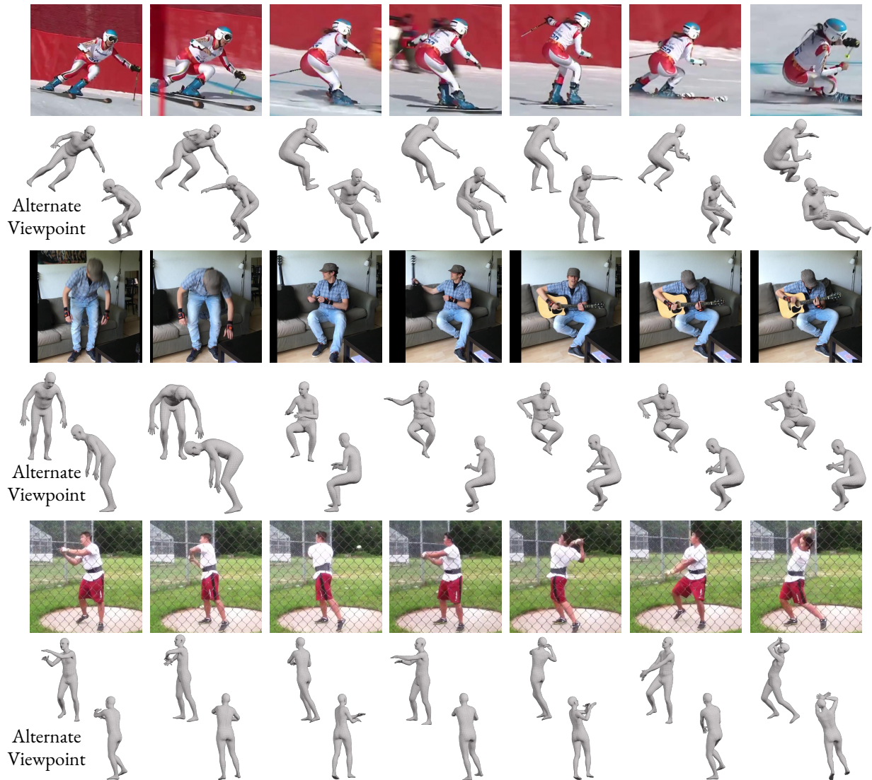
Figure 4: Qualitative results of VIBE on challenging in-the-wild sequences. For each video, the top row shows some cropped images, the middle rows show the predicted body mesh from the camera view, and the bottom row shows the predicted mesh from an alternate view point.
