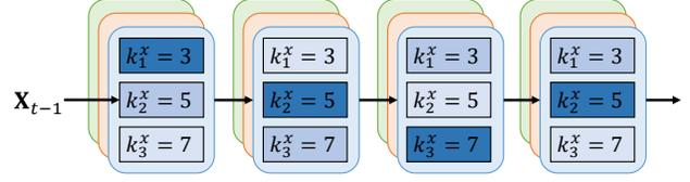
Figure 4. Illustration of multi-path kernel selection in one dimension. In this example, four AIC modules are stacked and for each module the kernel sizes for each dimension are  $\{3, 5, 7\}$ . The background darkness of the kernel indicates the value of the modulation factor, and thus reflects the selection tendency for this kernel. Stacking multiple AIC modules can increase the range of receptive fields exponentially.
