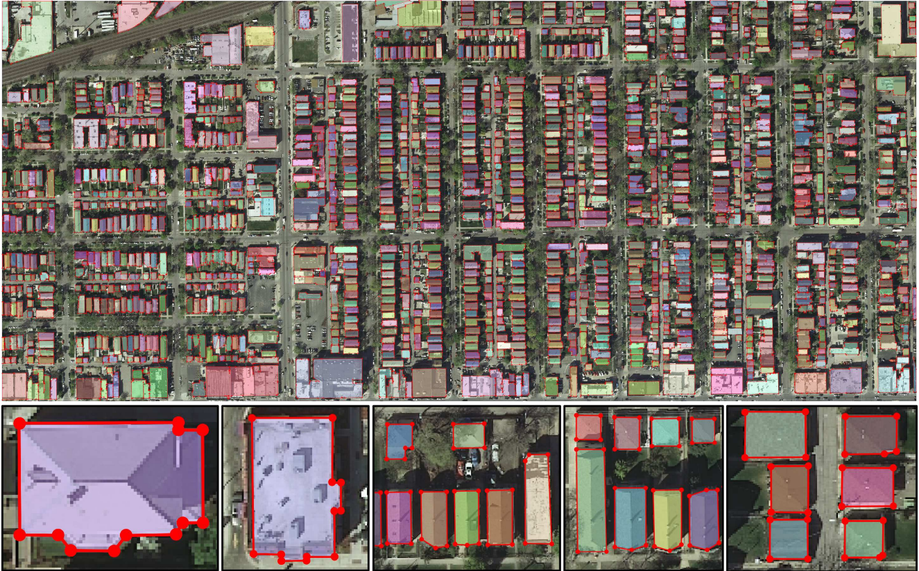
Figure 9. Extraction of buildings from satellite images with our algorithm: 1,178 buildings of a half square kilometer area of Chicago, USA, are extracted with low complexity polygons (8,683 vertices). While compact, the polygons capture some fine details (see closeups).
