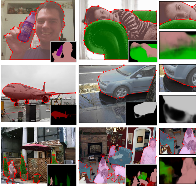
Figure 6. Vectorization of multi-class objects. Probability maps are often ambiguous and only roughly indicate the shape of the objects (see colors for different classes). Our algorithm captures the silhouette of these objects with low-complexity polygons with a good precision. Note in particular how the polygons nicely delineate close objects, such as the lady face and the couch (see close-ups). A failure case is shown in the bottom right example where the quality of the probability map is too poor to capture the underlying object. Images are from the PASCAL VOC2012 dataset.
