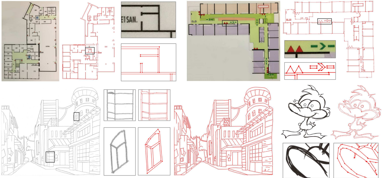
Figure 5. Vectorization of linear structures. Our algorithm can be used to vectorize floor map photographs (top) or line-drawings (bottom). While thin, these linear structures can be captured by compact polygons with a good accuracy (see closeups).
