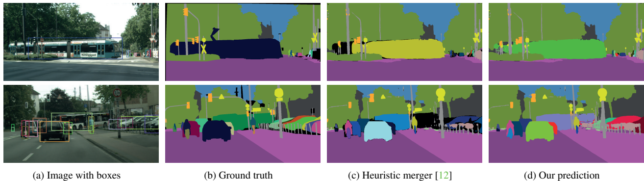
Figure 7. Qualitative results. The input images are shown with the predicted bounding boxes overlaid above. In column (c), swathes of “void” region are clearly visible for pixels where assignment cannot be made by heuristics. In contrast, our panoptic segmentation results are robust to incoherence in segmentation and localisation cues, and can explain more pixels in an image.
