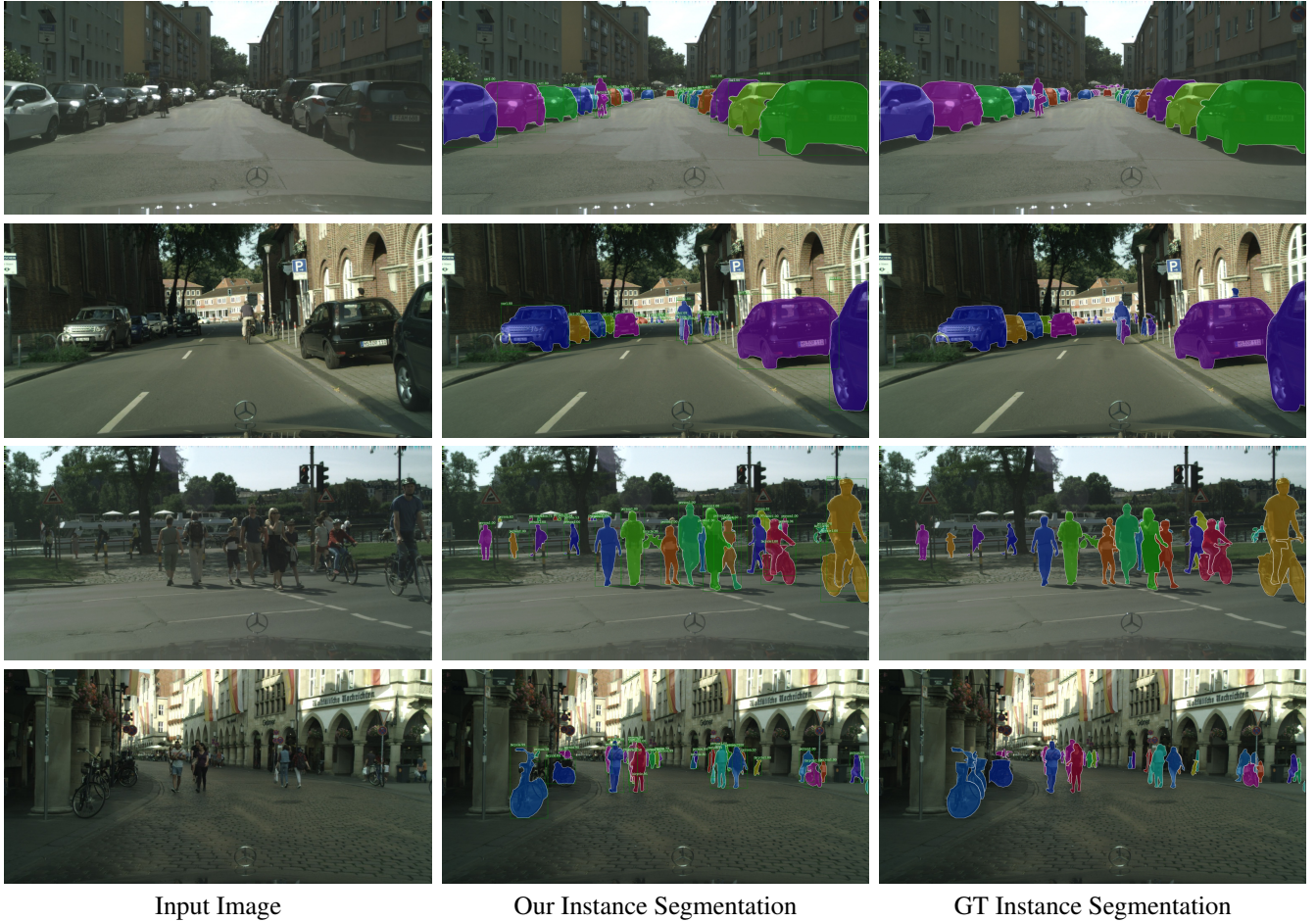
Input Image Our Instance Segmentation GT Instance Segmentation Figure 3. We showcase qualitative instance segmentation results of our model on the Cityscapes validation set.
