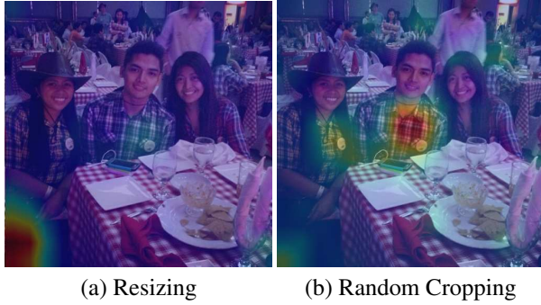
Figure 4. Resizing vs. random cropping as dataset preprocessing. This figure shows CAM heatmaps for an image from models trained with two preprocessing methods: (a) resizing and (b) random cropping. We observe that the resizing scheme learns cues in the edges or corners of images (note the focus on the lower left corner of (a)), where JPEG encoding can be asymmetric. On the other hand, the random cropping scheme captures the meaningful high-level cue—the chiral shirt collar.
