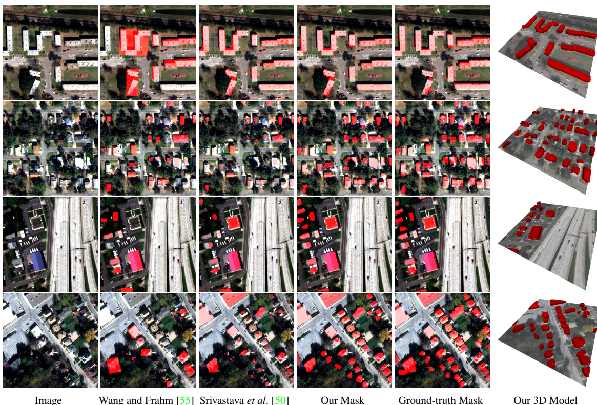
Figure 4: Comparison of building mask predictions for [55], [50], and our method. Right: Our 3D reconstruction.
