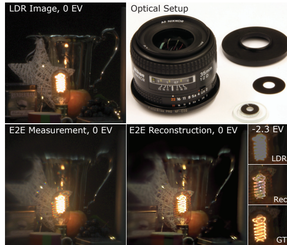
Figure 1: Conventional sensors are limited in their ability to capture high-dynamic-range (HDR) scenes. Details in brighter parts of the image, such as the light bulb, are saturated in a low-dynamic-range (LDR) photograph (top left). Our end-to-end (E2E) approach jointly optimizes a diffractive optical element (top right) and a neural network to enable single-shot HDR imaging. This deep optical imaging system records a single sensor image (bottom left) that contains optically encoded HDR information, which helps the network recover an HDR image (bottom right).
