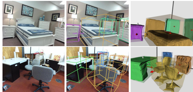
Figure 1: From a single image (left), we simultaneously predict the contextual knowledge including room layout, camera pose, and 3D object bounding boxes (middle) and reconstruct object meshes (right).
