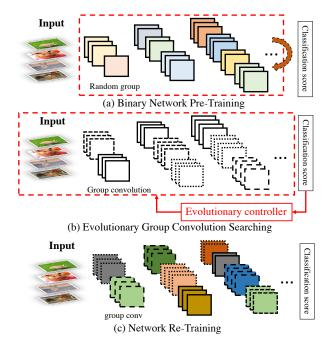
Figure 2. Framework overview of our proposed method. The process consists of three steps: train binary models with random groups (top figure, curve arrow indicates looping), apply evolutionary search to explore optimal groups based on accuracy metric, and re-train the searched group models from scratch.
