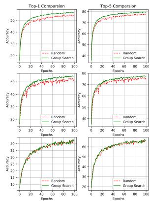
Figure 5. Validation accuracy on ImageNet through epochs of modified modules (M1, M2 and M3, from top to bottom respectively). Random: Groups are naively randomized for layers. Group search: Our proposed search optimal group architecture.
