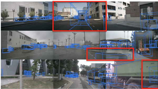
Figure 8. High PKL MEGVII mistakes MEGVII detections ranked most dangerous under the PKL metric. Most of the bottom ranked instances include false positives that are close to the ego vehicle.
