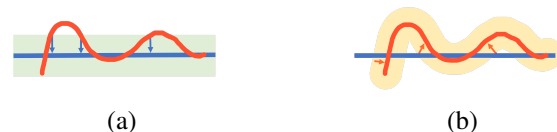
Figure 8. Occlusion boundary evaluation metrics based on the Chamfer distance, as introduced in [31]. The blue lines represent the ground truth boundaries, the red curve the predicted boundary. Only the boundaries in the green area are taken into account during the evaluation of accuracy (a), and only the yellow area are taken into account during the evaluation of completeness (b). (a) The accuracy is evaluated from the distances of points on the predicted boundaries to the ground truth boundaries. (b) The completeness is evaluated from the distances of points on the ground truth boundaries to the predicted boundaries.
