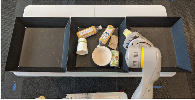
(a) Single-bin grasping evaluation setup: All robots are placed in front of the center bin, which contains all the 6 objects.
