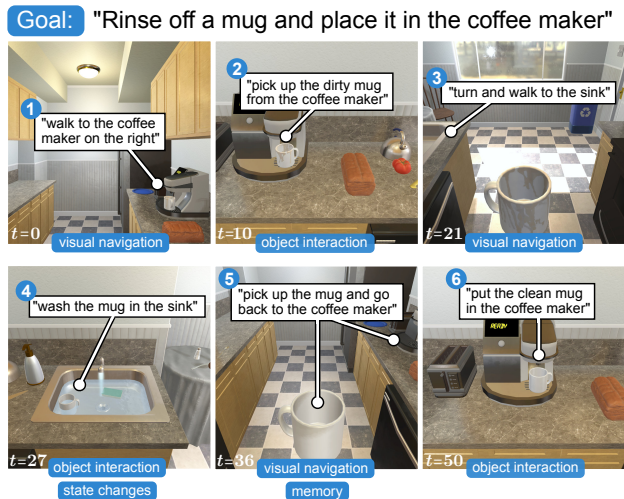
Figure 1: ALFRED consists of 25k language directives corresponding to expert demonstrations of household tasks. We highlight several frames corresponding to portions of the accompanying language instruction. ALFRED involves interactions with objects, keeping track of state changes, and references to previous instructions.
