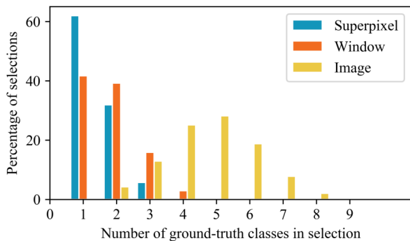
Figure 8: Distribution of number of unique ground truth classes in selections made by different approaches. The majority of the selections made by our superpixel approach have only a single ground truth label in them. Compared to the fixed window approach which has an expected 1.83 unique classes per selection, our approach has 1.40 expected classes per selection. Here, the average number of pixels per window and per superpixel was taken to be the same.
