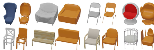
Figure 17: Test set chair CSG abstractions. We predict eight rounded cuboids minus eight other rounded cuboids.
