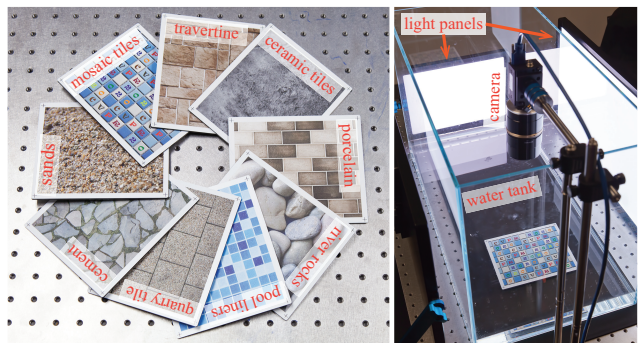
Figure 8. Our experimental setup for real data acquisition. Left: Sample reference patterns that we use for the real experiments; Right: We setup a camera on top of the fluid tank to capture refraction images of the reference pattern.
