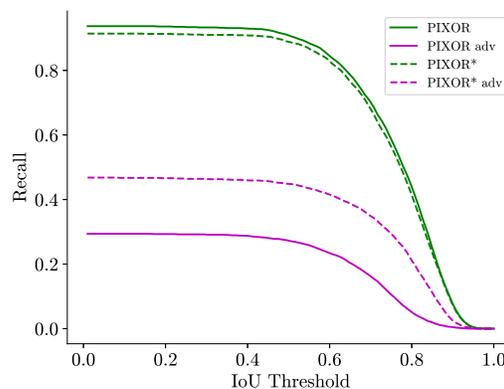
Figure 8: We perform our attack on two similar models. PIXOR converts the input point cloud to occupancy voxels and PIXOR\* separates points into columns and extracts features with a pointnet backbone. Although the models have the same backbone architecture, PIXOR\* is significantly more robust due to the input representation.
