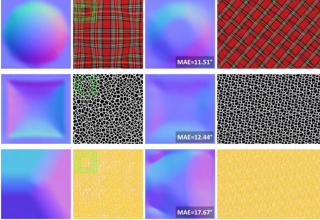
Figure 5: Shape and texture results for synthetic images. From left to right: surface normals of the true shape; input image; output surface normals (with MAE); and sample from output texture generator. Green inset squares show patch sizes used by the unwarper.
