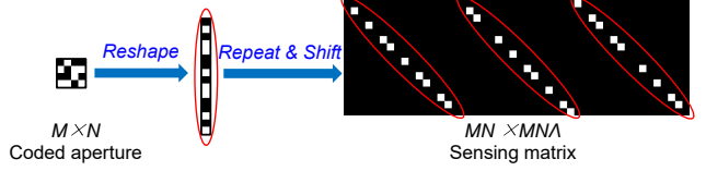
Figure 3. The transition from the coded aperture to the sensing matrix. To synthesize the block diagonal sensing matrix, the coded aperture is first reshaped as a vector, then repeated in the horizontal direction, each time with a uniform shift in the vertical direction, as many times as the number of spectral band.
