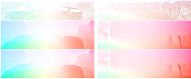
Figure 5. Examples of ground truth ( top ), HD3 optical flow ( middle ), and PPAC-refined optical flow ( bottom ) on KITTI. Best viewed on screen.
