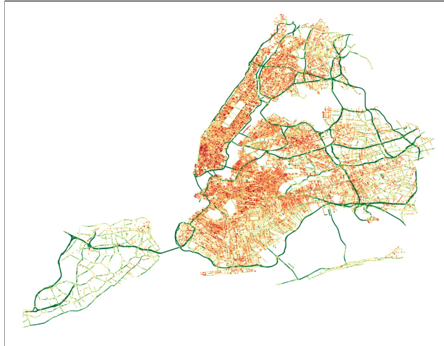
Figure 3: Example traffic speed data from Uber Movement Speeds for New York City (visualized as free-flow speeds for January 2018).
