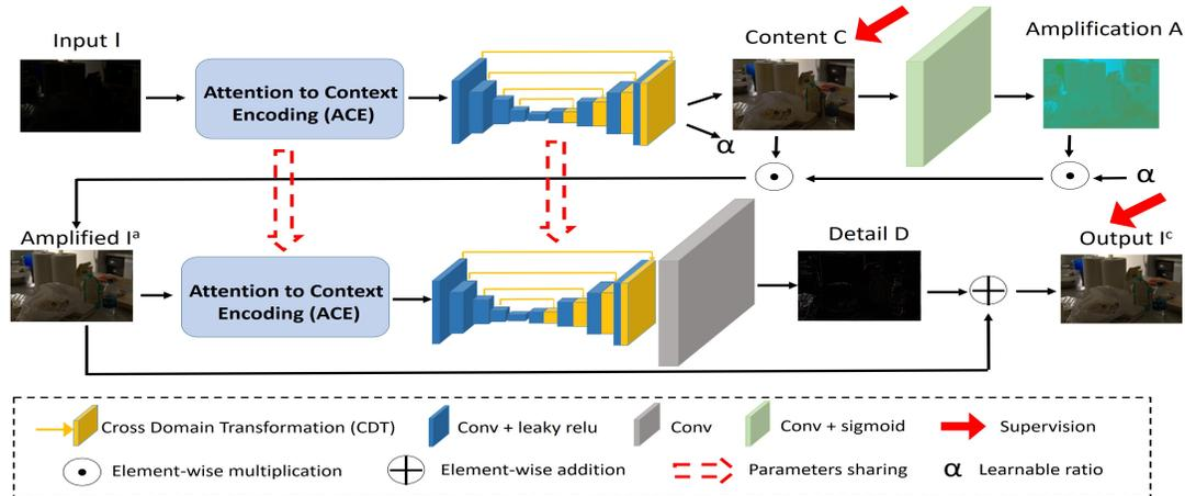
Figure 3. Overview of the proposed model. In the first stage, the network enhances the low-frequency contents of input image  $I$  with noise suppressed, and then amplifies it to produce  $I^a$ . In the second stage, the network infers the high-frequency details from  $I^a$  to produce the output enhanced image  $I^c$ .
