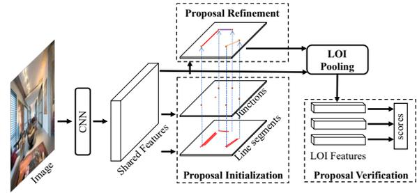
Figure 2. Illustration of the architecture of our proposed HAWP. It consists of three components, proposal initialization, proposal refinement and proposal verification. See text for details.
