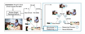
Figure 1. Scene Graph guided Modular Network (SGMN) for grounding referring expressions. SGMN first parses the expression into a language scene graph and models the image as a semantic graph, then it performs structured reasoning with neural modules under the guidance of the language scene graph.
