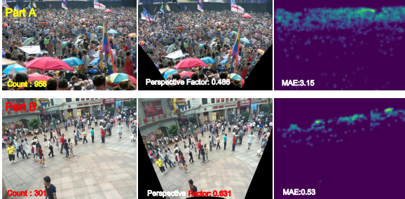
Figure 10: Examples in ShanghaiTech dataset. The first column is the input images, and the second column is the warped images, while the third column is the estimated density maps. The proposed method adaptively warps the images and delivers accurate estimations.
