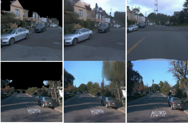
Figure 5. Novel View Synthesis. The first column is Surfel image under novel view, the second column is our synthesized result. The third column is the original view. Additional visualization can be found in Supplementary Sec. B.
