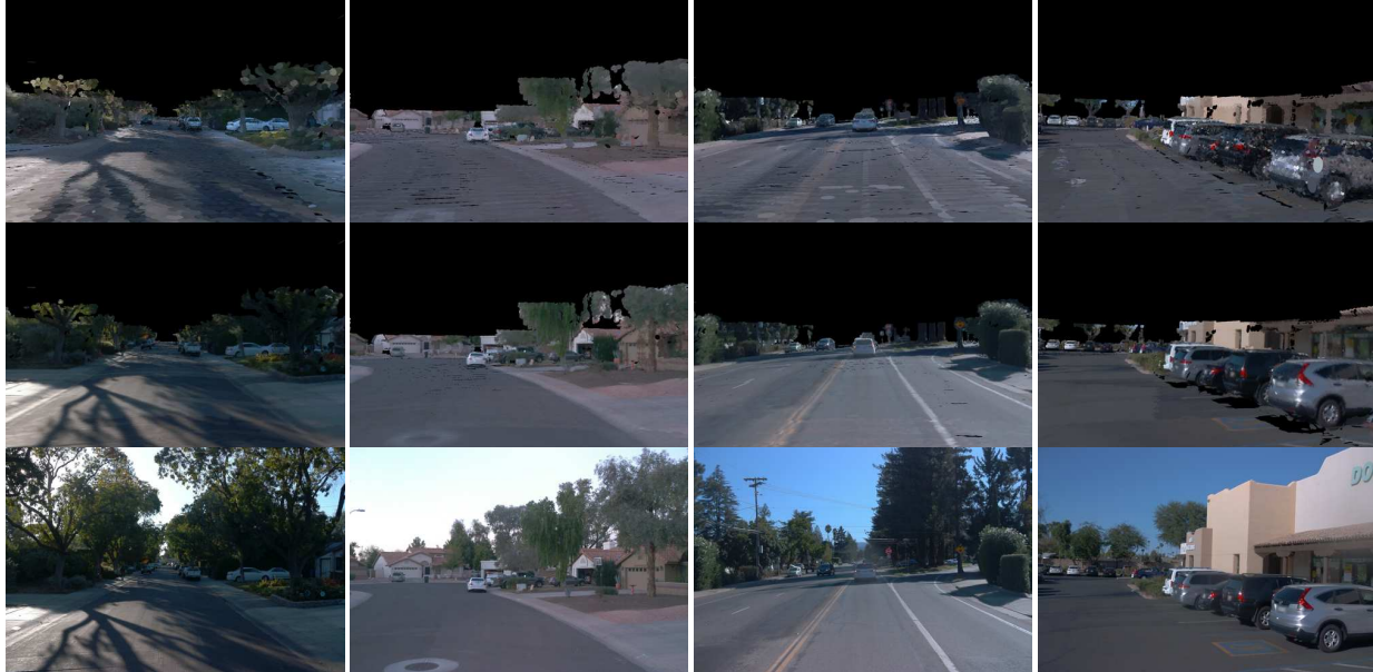
Figure 2. Visualization of different scene modeling strategies. Top row : Surfel baseline; Center row : our Texture-Enhanced Surfel Map (also known as surfel rendering in the rest of the paper); Bottom row : Real camera image.
