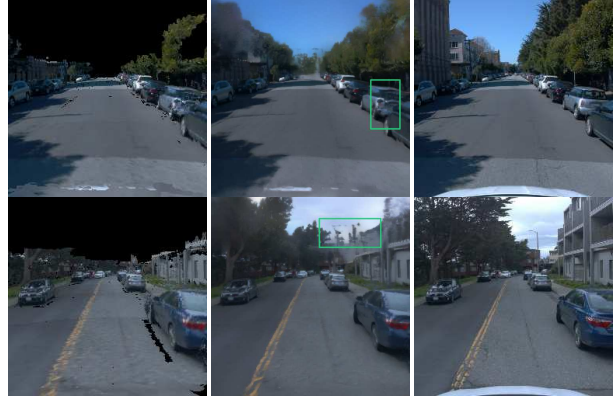
Figure 6. We show two typical failure cases, the first is the case where reconstructed Surfel map contains too large errors. The second is on the unmapped region (top part of building in this example).
