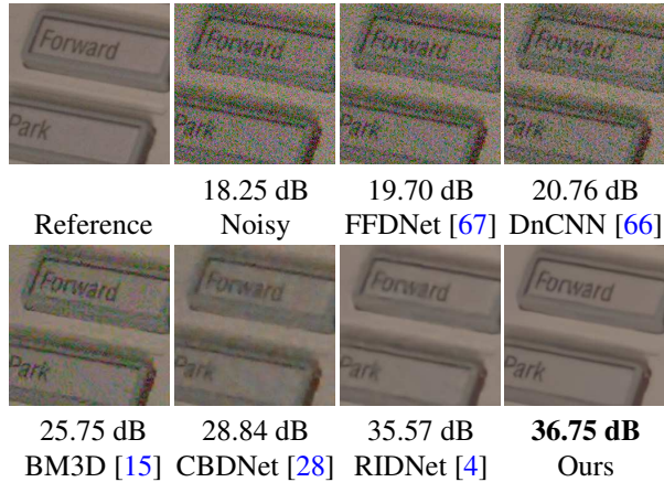
Figure 7: Denoising results of different methods on a challenging sRGB image from the SIDD dataset [1].
