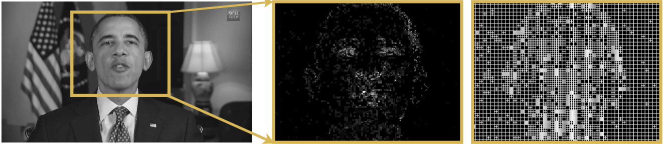
Figure 6. The illustration of encoder information of the H.264 video compression standard. Left : prediction frame in Y channel. Middle : prediction residual image in Y channel. Right : transform unit (TU) partition.
