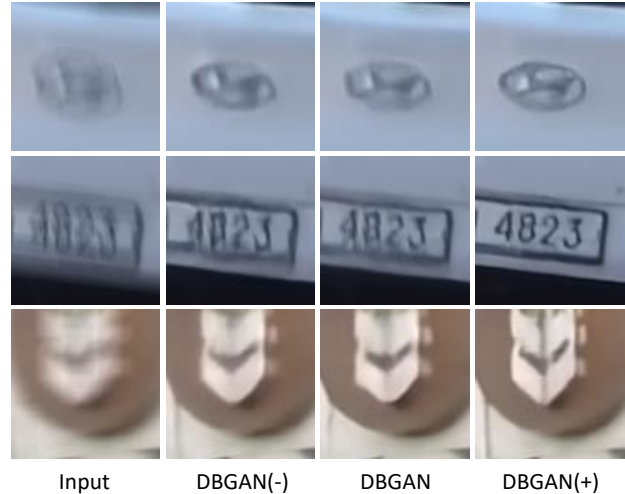
Figure 5. Qualitative ablation results. Examples of deblurred images generated by the proposed framework with different model structures. The first column shows input blurred images, and the next three columns are the deblurred images produced by DBGAN(-), DBGAN and DBGAN(+), respectively.
