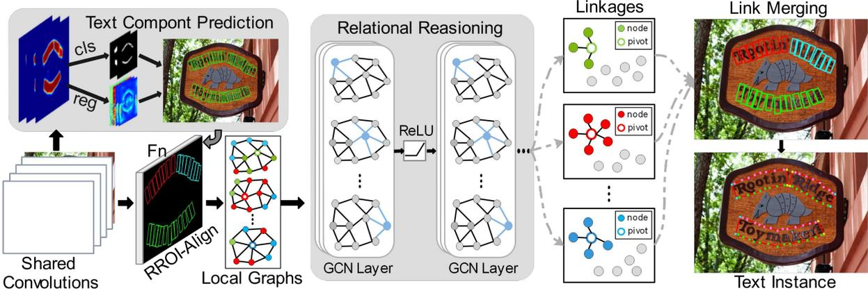
Figure 2. Overview of our overall architecture. Our network mainly consists of five components, *i.e.*, shared convolutions, text component prediction, local graphs, relational reasoning, and link merging.
