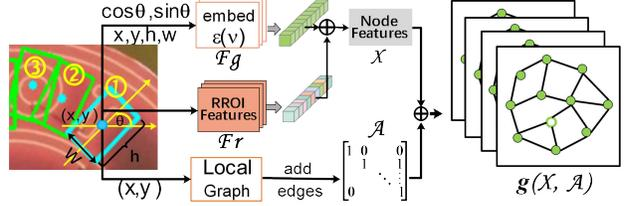
Figure 5. Illustration of  $g(X, A)$  generation.  $F_r$  represents the geometry features;  $X$  is node feature matrix;  $A$  is an adjacency matrix;  $g(X, A)$  represents the mathematical expression of local graph. The details of embedding operation in Eq. 12 and Eq. 13.
