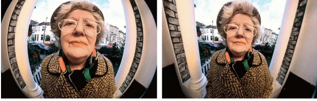
Figure 2. Left: An image of a woman standing in front of the access control system. It suffers severe radial distortion [source: Google Images]. The distortion will degrade the performance of previous face recognition systems. Right: Image corrected by the proposed method.
