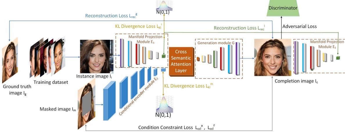
Figure 2: Overview of our architecture with two branches. The primary branch consists of a manifold projection module and a generation module, which is responsible for mapping the instance image space to the conditional completion image space. The secondary branch consists of a conditional encoder module, which acts as the conditional label.
