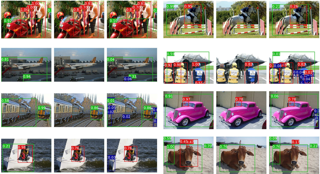
Figure 3. Visual examples of our ZSD results. Each triple shows: (from left to right) DELO detection results, vanilla YOLOv2 detection results at the same confidence threshold as DELO, vanilla YOLOv2 detection results at a much smaller confidence threshold. The seen, unseen and errors are color-coded as red, green and blue. Notice that compared to DELO, the vanilla YOLOv2 constantly predicts extremely low objectness scores on unseen objects, and suffers from significant detection errors for those unseen objects to be detected.
