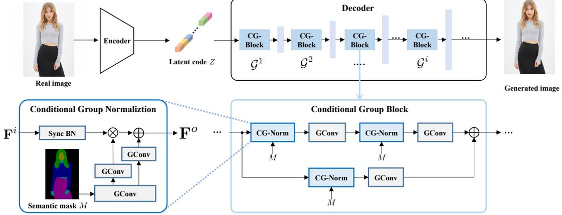
Figure 2: Architecture of our generator (GroupDNet). “GConv” means group convolution and “Sync BN” represents synchronized batch normalization.  $\mathcal{G}^i$  is the group number of  $i$ -th layer. Note normally  $\mathcal{G}^i \geq \mathcal{G}^{i+1}$  for  $i \geq 1$  for GroupDNet.
