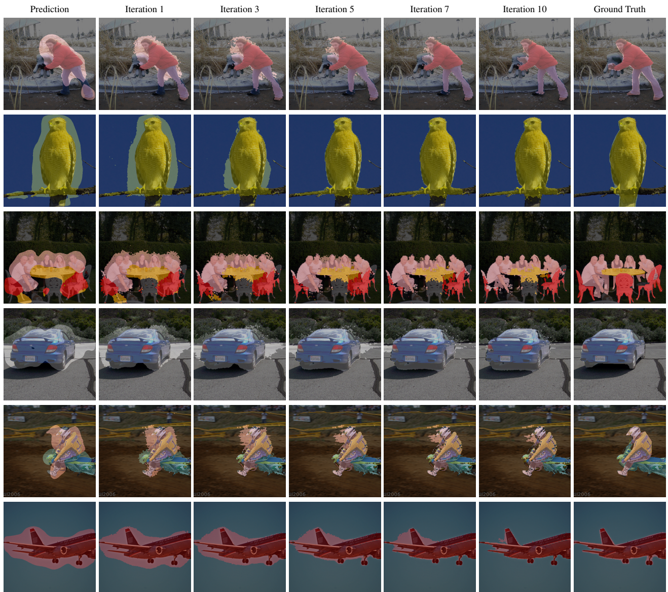
Figure 10. Visualisation of PAMR iterations. The initial model predictions suffer from local inconsistency: mask boundaries do not align with available visual cues. Our PAMR module iteratively revises the masks to alleviate this problem. Our model uses the mask from the last iteration for self-supervision.
