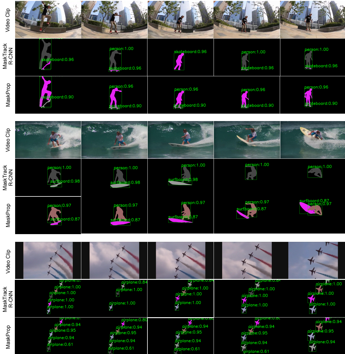
Figure 1: We compare our video instance segmentation results with those produced by MaskTrack R-CNN [5]. Different object instances are shown with different colors. The first row for each video shows the original frames. The second row illustrates the mask predictions of MaskTrack R-CNN and the third row those obtained with our MaskProp. Compared to MaskTrack R-CNN, on these sequences our MaskProp tracks object instances more robustly even when they are occluded or overlap with each other.
