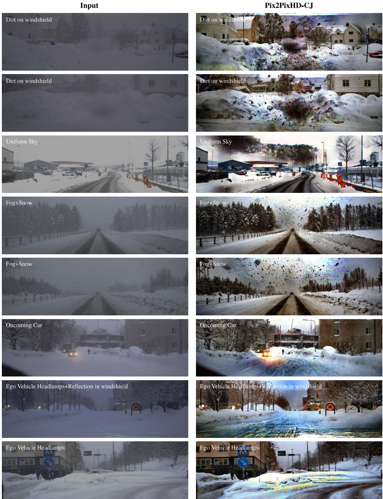
Figure 27: Failure cases for image reconstruction methods on unseen distortions. The learned distortion removal models were only trained on synthetic foggy scenes and therefore have limited generalization capabilities as different disturbance types can occur in combination as snow and fog.
