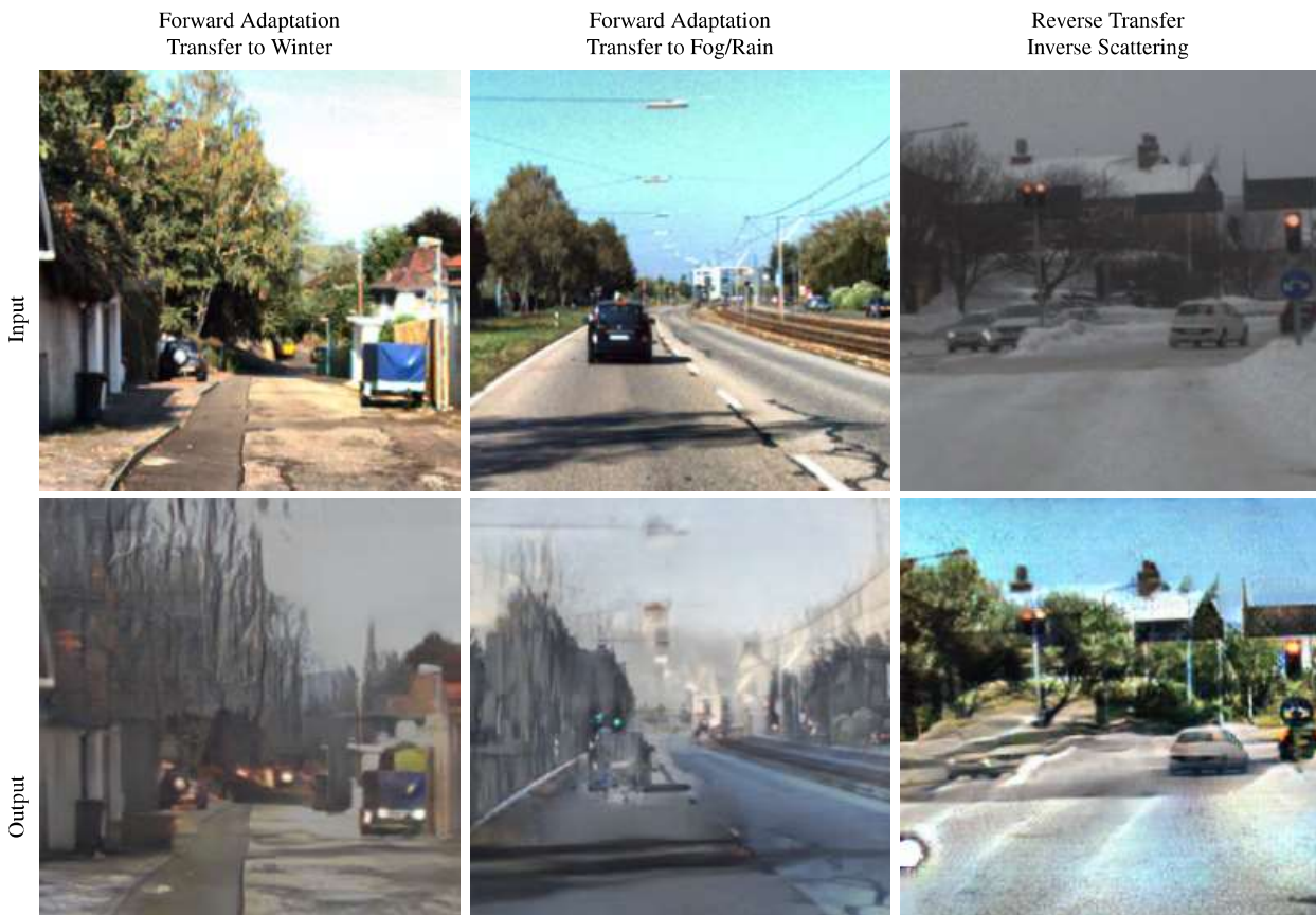
Figure 18: Examples for domain adaptation using CyCADA[9]. Adapting KITTI (left) to our experimental data adapts to winter scenes with snow, but does not properly model fog distortions (middle). For completeness, (right) shows a reverse transfer. The reverse transfer does not recover enough information to model a clear scene correctly.
