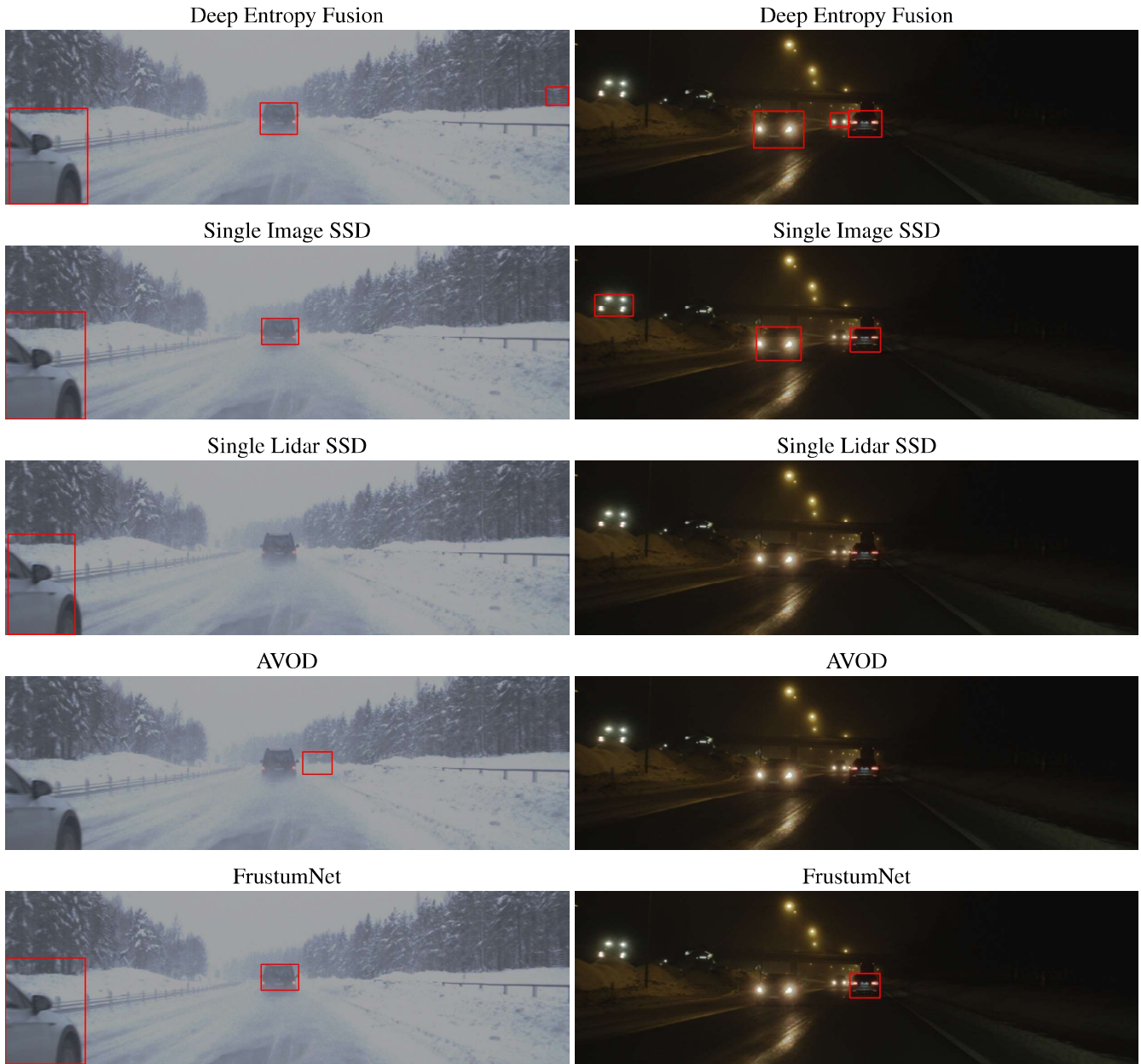
Figure 16: Additional qualitative detection results for in-the-wild measurement distortions that have not been seen during training. The left column shows disturbances through spray and an incorrect auto exposure, the right column show detections in during fog and nighttime.
