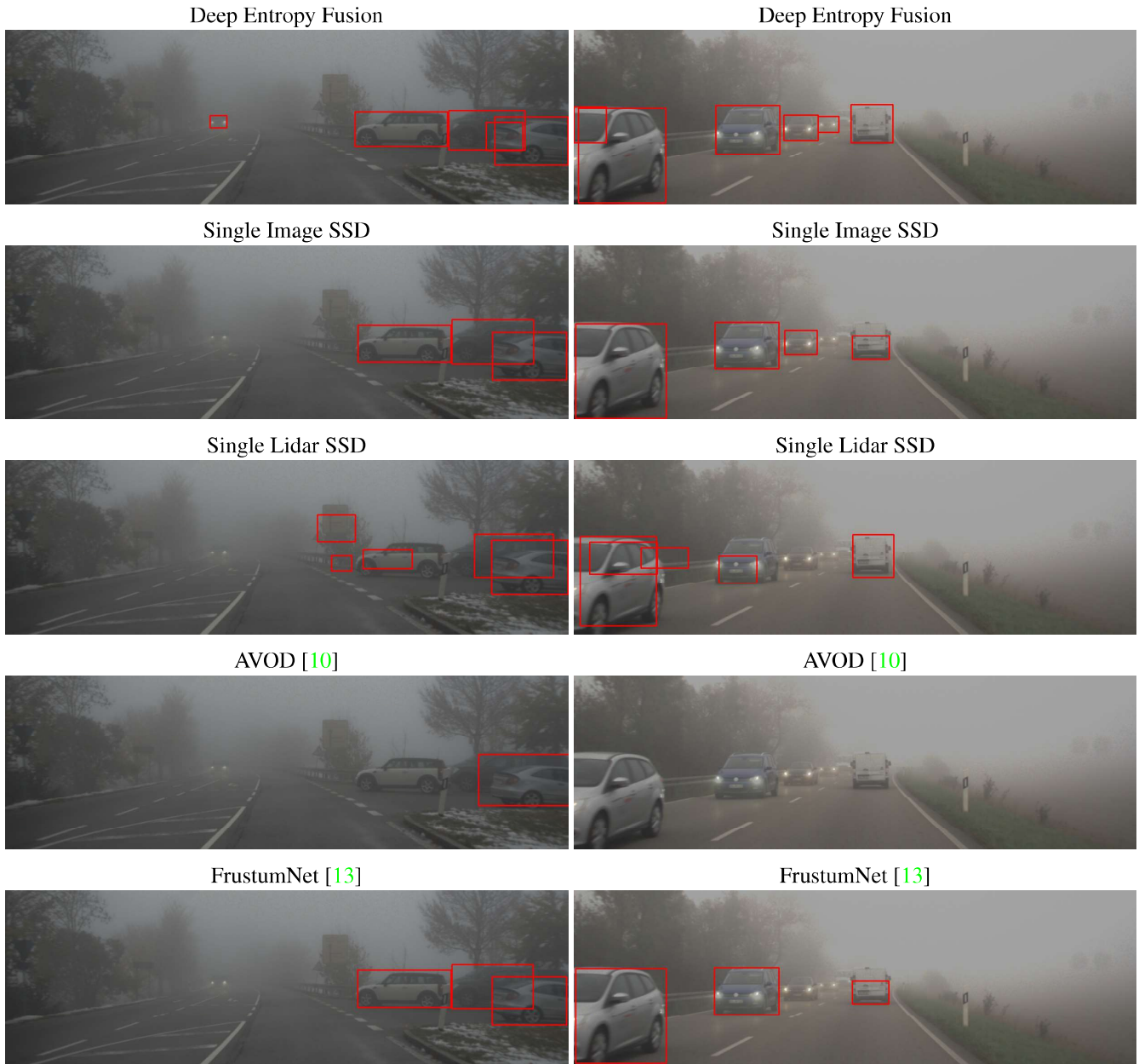
Figure 13: Additional qualitative detection results for in-the-wild measurement distortions that have not been seen during training. The left and right columns show disturbances in dense fog in different illumination settings on a suburban road.
