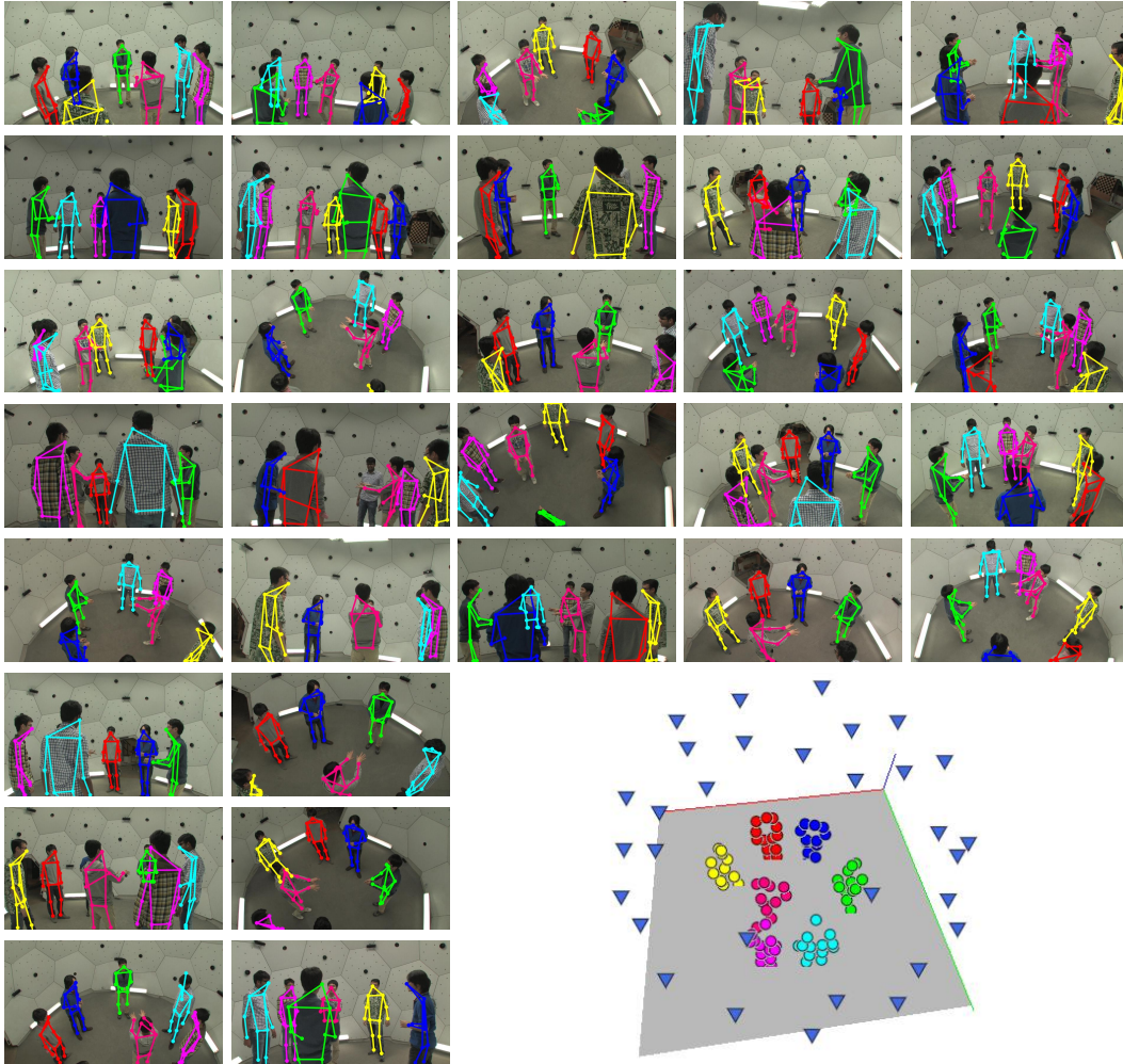
Figure 4: Qualitative result on the CMU Panoptic dataset. There are 31 cameras and 7 people in the scene. The cameras are distributed over the surface of a geodesic sphere. As we detailed in ablation study, with the proposed iterative processing all the 31 cameras can be updated in around 0.058 seconds.
