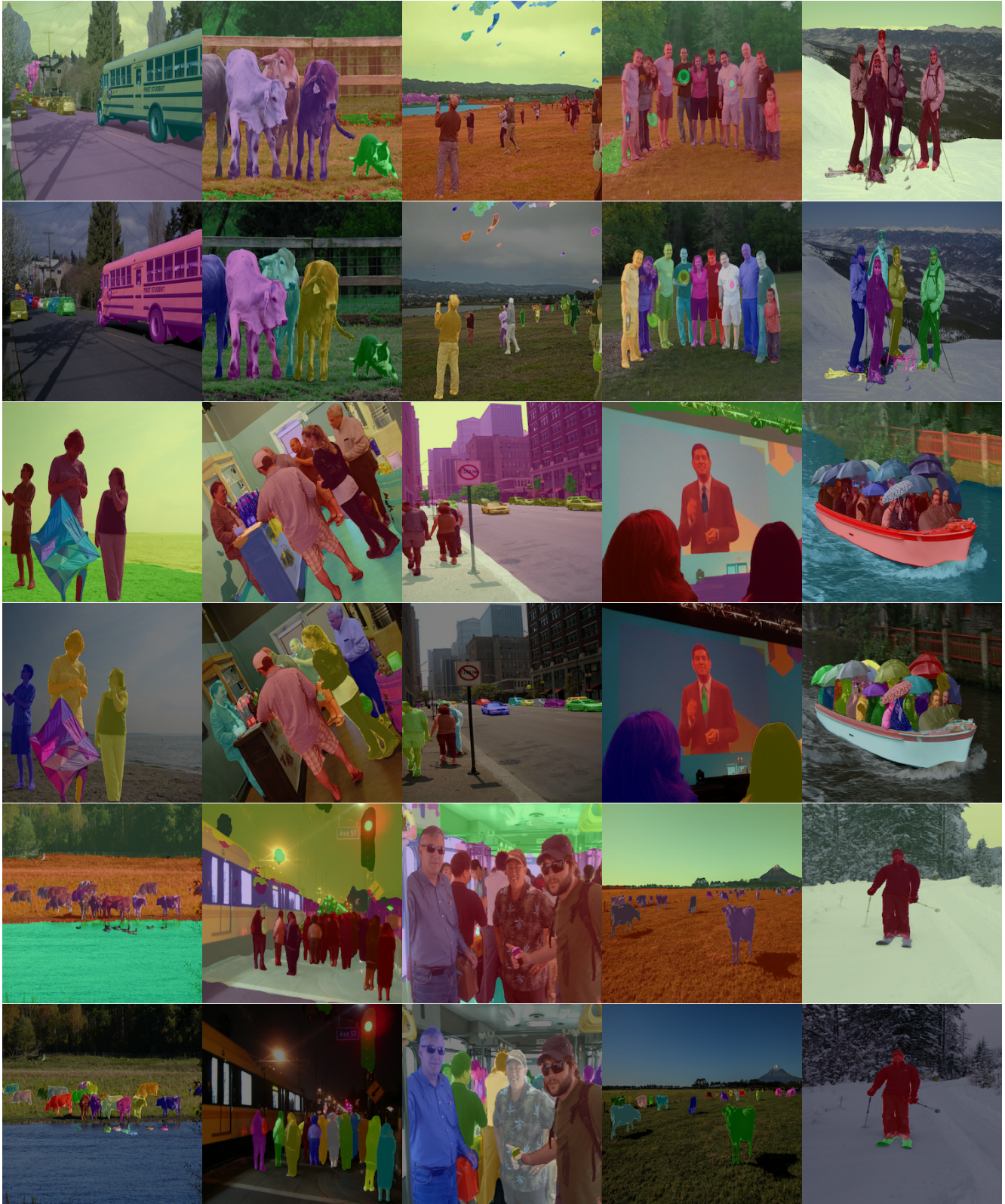
Figure 7. Visualization of Panoptic-DeepLab with Xception-71 on COCO val set. Only single scale inference is used and the model achieves 39.7% PQ. The first row is panoptic prediction and the second row is instance prediction.
