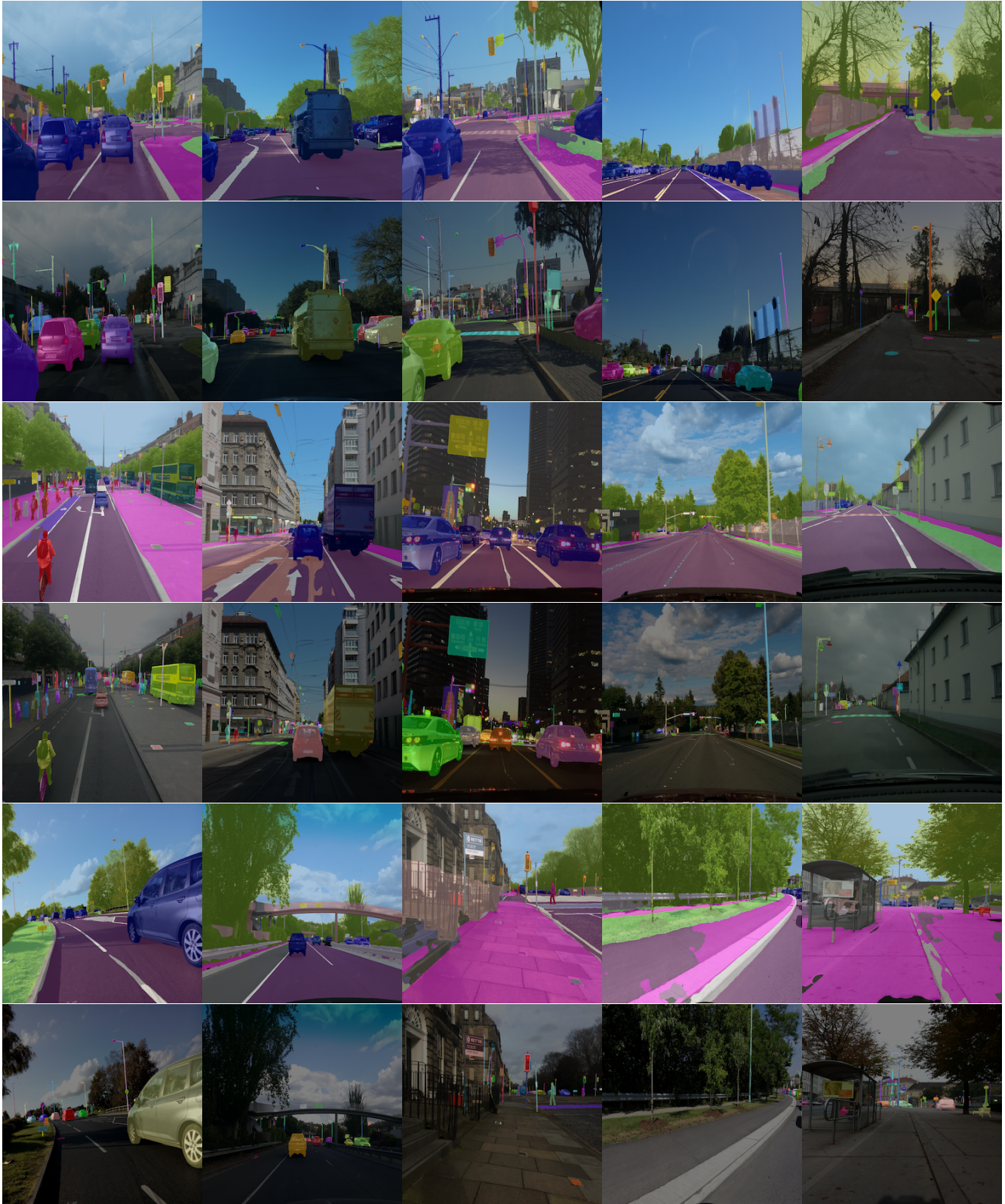
Figure 6. Visualization of Panoptic-DeepLab with Xception-71 on Mapillary Vistas val set. Only single scale inference is used and the model achieves 37.7% PQ. The first row is panoptic prediction and the second row is instance prediction.
